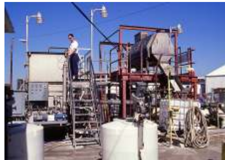
200 GPM Beef Further Processing Phys/Chem System
