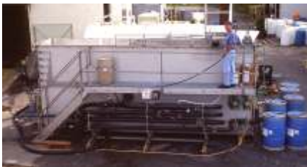
Complete skid-mounted 200 GPM Phys/Chem System with LS Reuse Option at an industrial laundry includes 1,068 Gal. effluent holding compartment, flotation chamber, sludge holding compartment, polymer holding tanks, all pumps, all valves, all piping and is pre-wired and tested at the factory.
