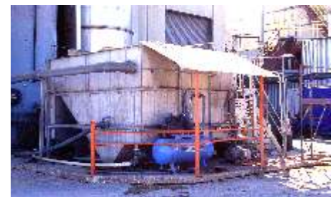
600 GPM Phys/Chem System - Meat Packing and Rendering
